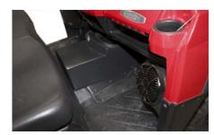
Once the enclosure is in place, screw the 6 mounting screws into the floor using a phillips screw bit in a cordless drill
