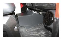
Place the enclosure on the passenger side footwell and lift the box onto the center hump, lift the driver side higher and slide in using a sidways motion
